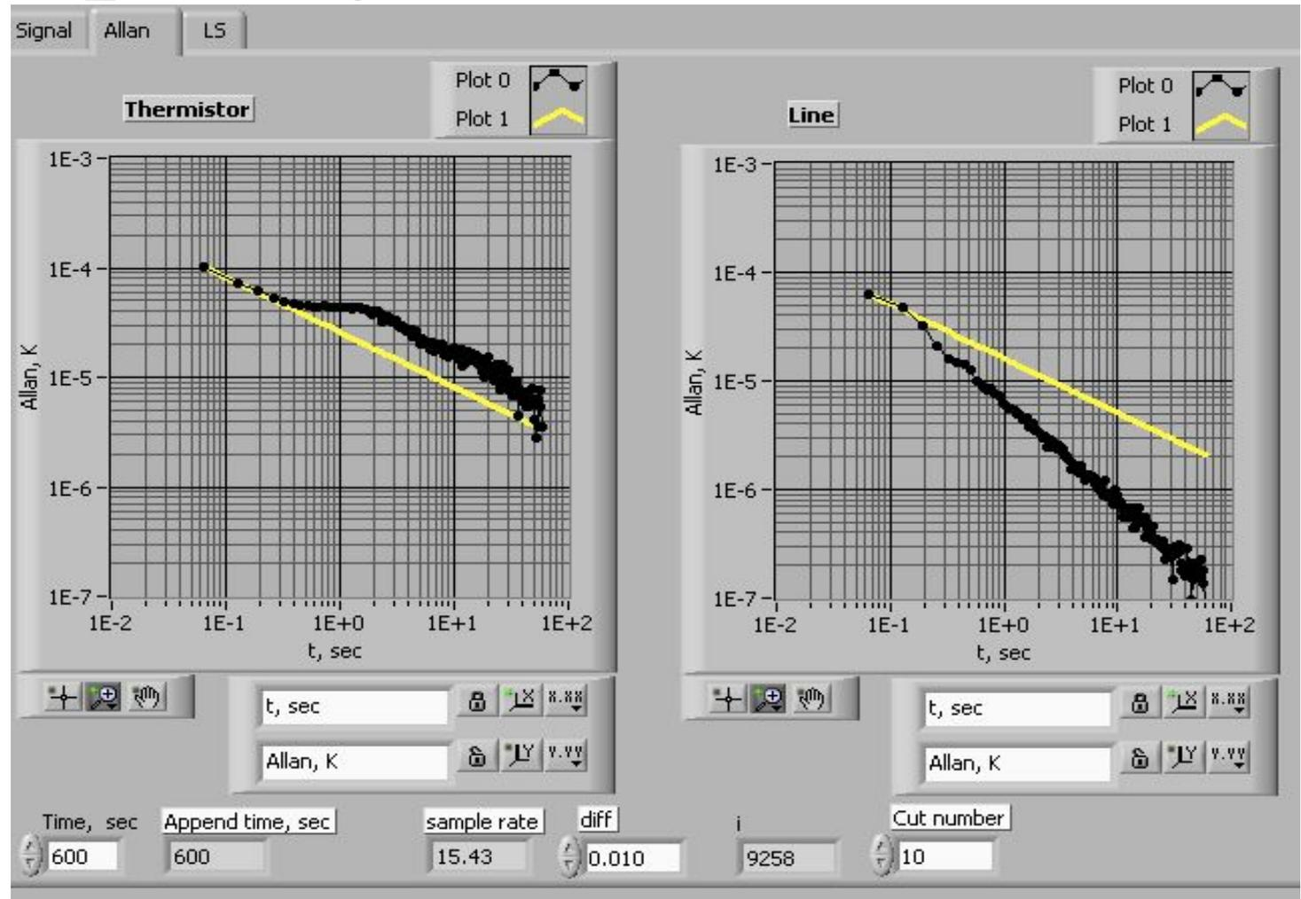
Allan plot of temperature as measured by termistor (left) and using spectral line (right). Both temperature stabilization and frequency tuning cycles stabilization were on.
