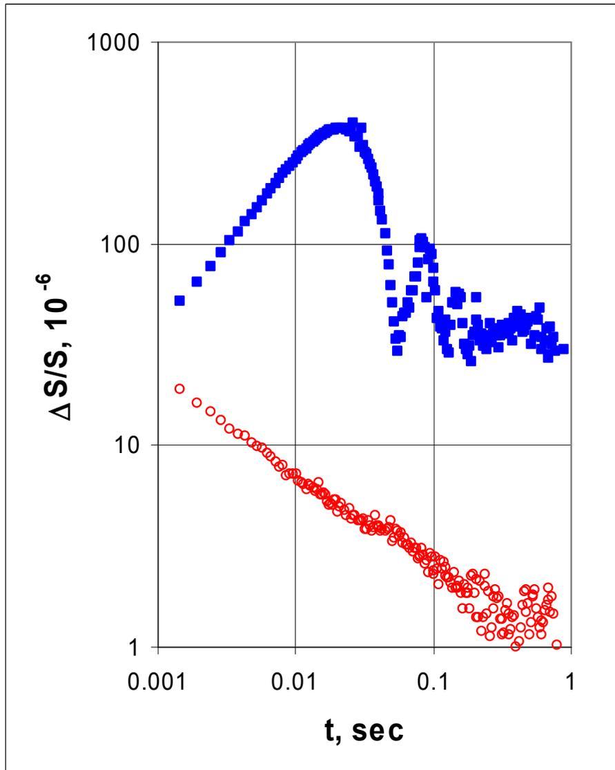
Harmonic modulation of relative signal (solid blue squares) due to generated mechanical vibrations in optical setup. Flicker type noise of DL radiation at  $3 \cdot 10^{-5}$  level can also be observed.
