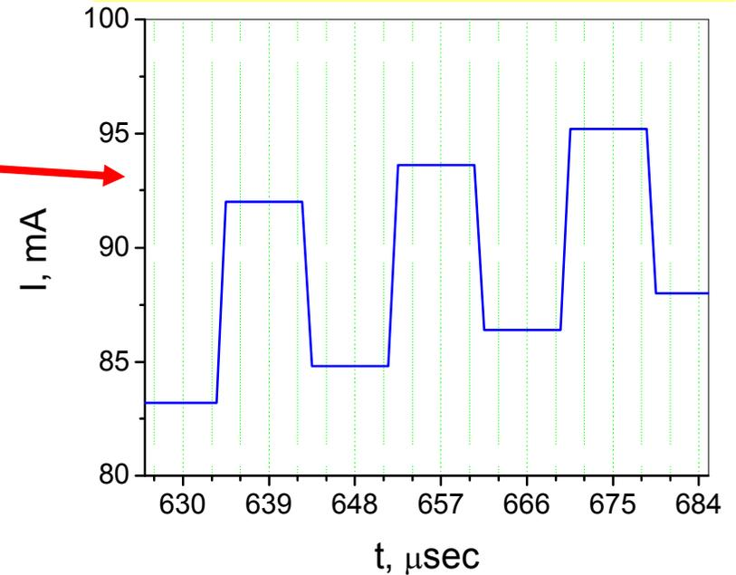
Most typical excitation current waveform in use: "0" – current below threshold value;  $N = 3-10000$  (100 in present case). Modulation is important component.
