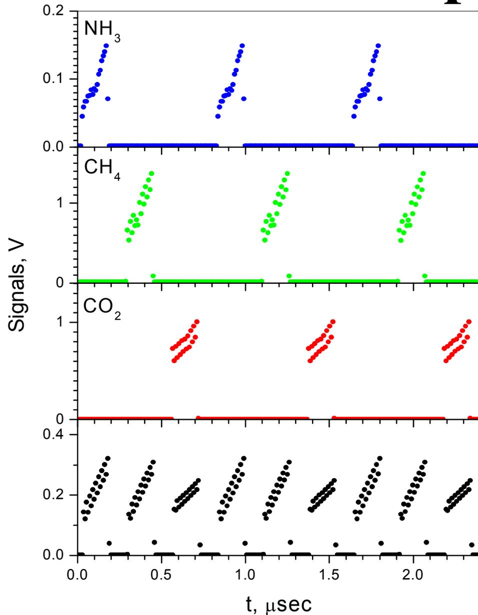
For time multiplexing regime, excitation current generated by PC can be presented as matrix in  $N \times M$  dimensional space.
