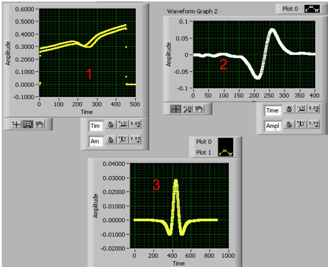
Hence, optimal signal filtering is cross-correlation function of recorded absorption derivative in reference channel with analytical one.
