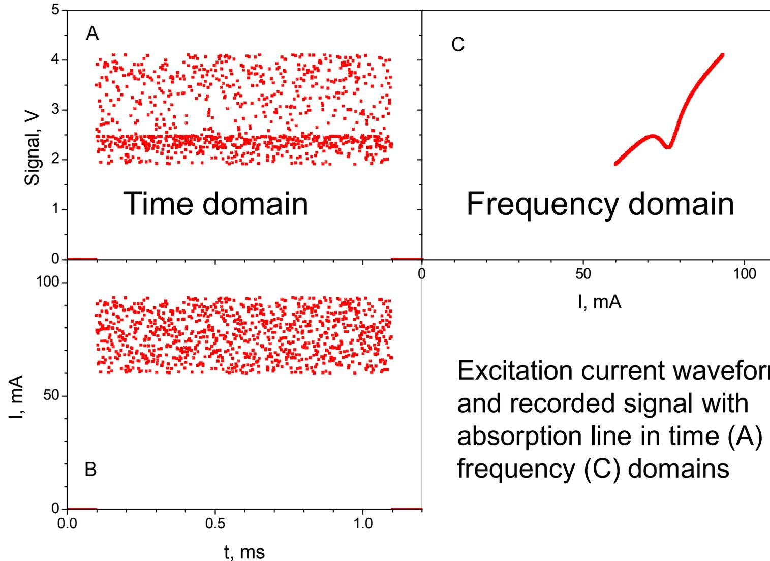
Excitation current waveform (B) and recorded signal with absorption line in time (A) and frequency (C) domains
